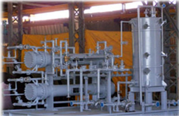
Aux. Skid packaging -Cooling water console Client - Dresser rand End User- Inelectra- Colombia
